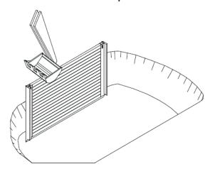
After measuring of the trench, initial excavation for the shaft is done, depending on the panel lengths used, according to the instructions of the construction supervisor and the applicable DIN standards.
