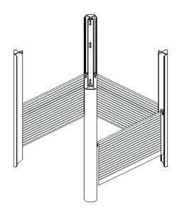
Alignment of the shoring is required so that the last shoring wall can also be positioned without any problems. To this end, the clear distance between the shoring panels at both ends of the panels on the one hand and the measurement across the two diagonal axes of the shoring field on the other must match.
