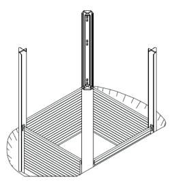
Once the fourth base panel has been positioned, the angularity of the shoring must be checked again. The cavity between the soil and the shoring panel must then be backfilled and compacted.
