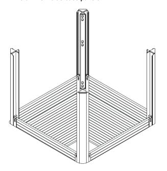
The inside base panels are swiveled between the guide frame in accordance with image a), guided into the U-shaped guide rails on the outside panels and lowered to the bottom of the trench. Further trench excavation is done through lowering of the inside base panels and the guide supports
