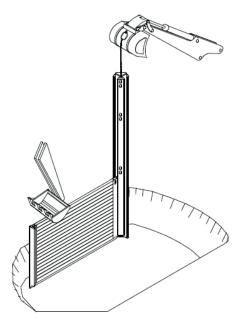
The corner rail can be swiveled in with the help of a second hoist (see images a, b, c) or pushed over from above. Care must be taken here to ensure that the rear square of the corner rail (1) catches behind the square of the shoring panel (2).
