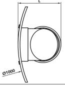
The indicated distances in the drawing are needed for the three different versions of the ILA. For the Funke-ILA 160 the distance from the chamber wall is just 217 mm, for example. This provides a non-restricted chamber accessibility.
