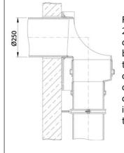
For the Funke-ILA 250 version, the dowpipe is going to be connected with the help of a reducer 250/200 (included in the scope of delivery) as shown in the drawing on the left.
